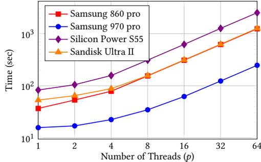
**Figure 1: Time to read 10GiB per thread on each SSD tested. The DAM model predicts that the time would increase linearly with the number of LBAs read. However, for a small number of threads the time stays relatively constant.**
