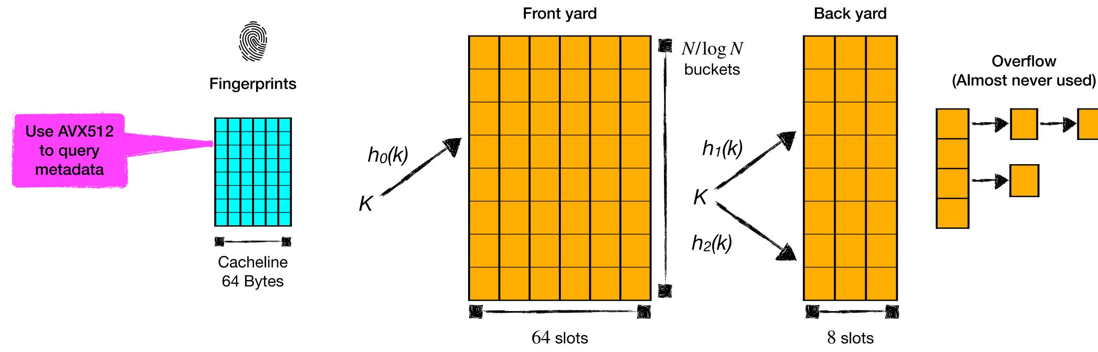
**Problem:** buckets in the front yard span many cache lines, so queries must load many cache lines.
