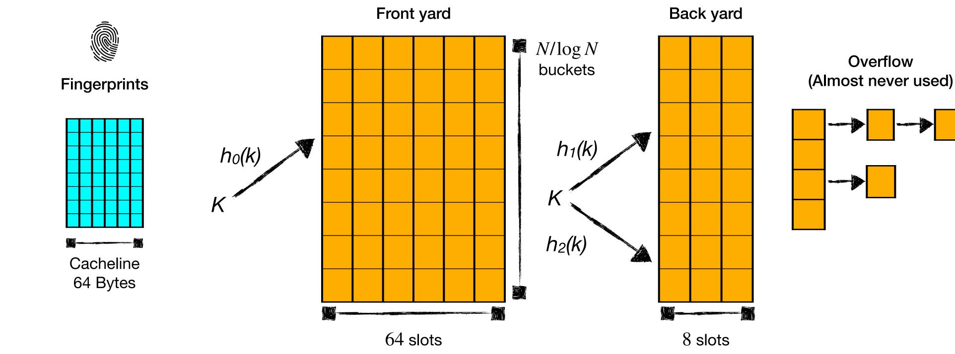
**Problem:** buckets in the front yard span many cache lines, so queries must load many cache lines.
