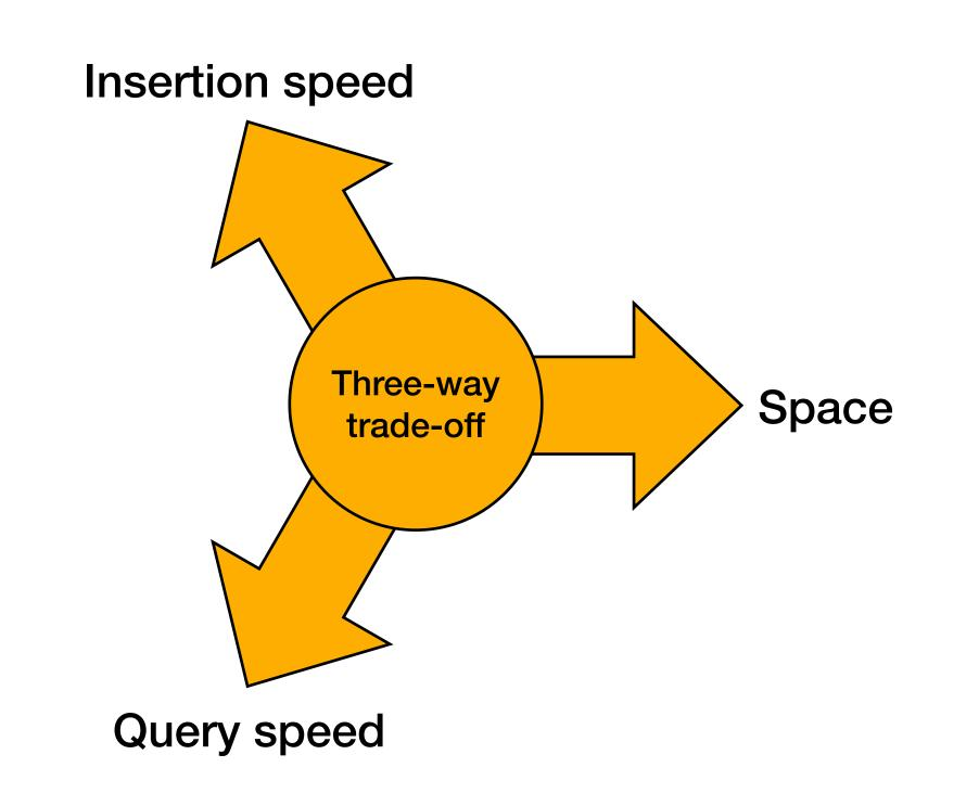
Hash table performance has a three-way trade off between insertion speed, query speed, and space.
