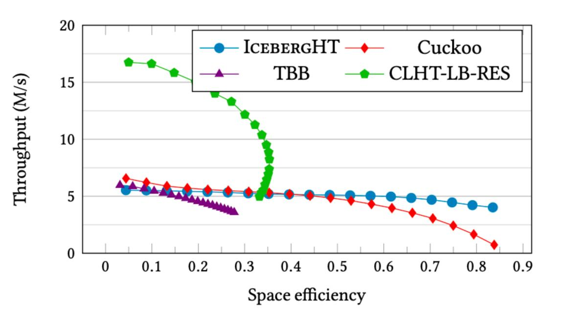
IcebergHT can achieve high space efficiency and maintain insertion throughput. CLHT space efficiency drops quickly. CuckooHT insertion throughput drops at high load factor.
